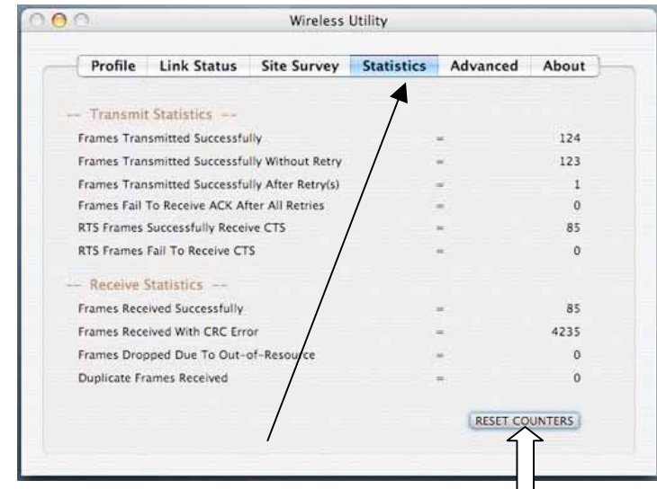
The STATISTICS screen keeps count of transmit statistics & receive statistics with a RESET COUNTERS button at the bottom to clear and restart the count over.
